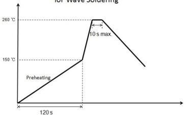
Notice: Wave Soldering is suitable for 1206 and 0603 size.
